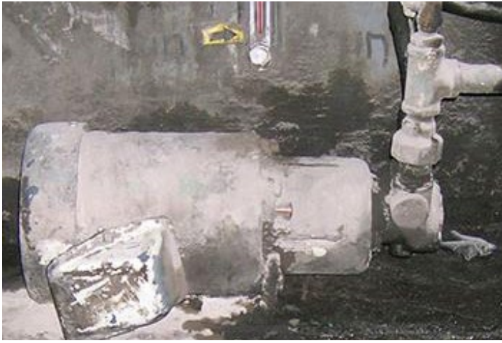
Machines that are not kept clean or that operate in dirty environments can ingest a significant amount of contaminants.
